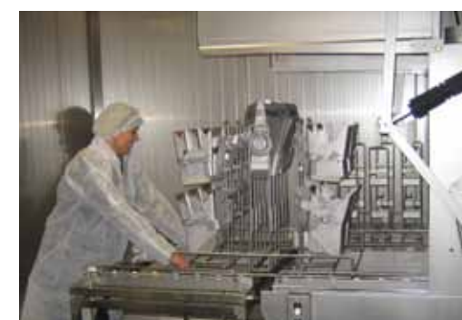
Push the rack into the utensil washer for cleaning.
