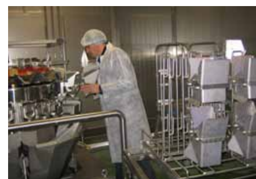
Load/unload the scale part directly at the weighing unit.
